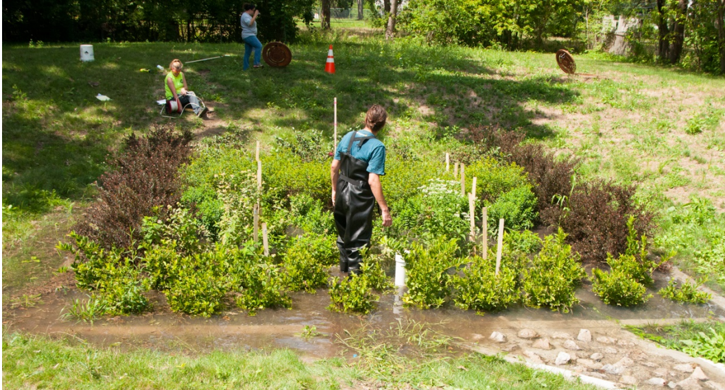
Figure 2 Flood Test to Monitor Performance Including the Drain Time
