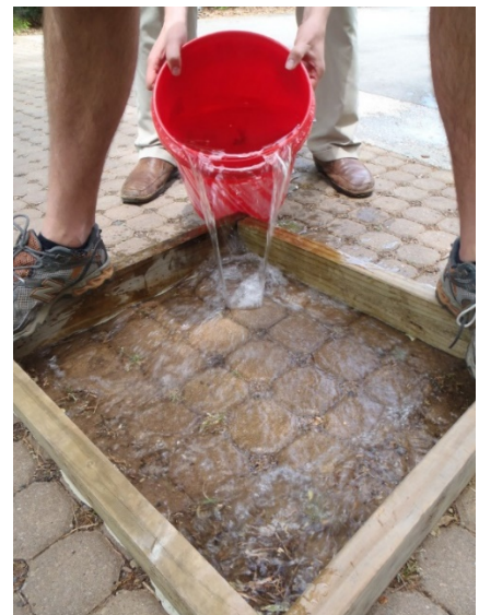
Figure 13 Simple Infiltration Test
